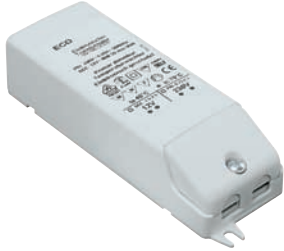
P 97772N ECO Transformator 80VA weiß / white 230/12V, max. 20-80W 125x38x28mm
